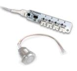
The X-Touch button interface is a 4-channel pushbutton interface with LED control and can be used in combination with industry-standard push buttons. It allows the connection of up to four buttons onto a single interface. This results in the connection possibility of up to 9 push buttons even on the smallest Xperience Controller. Programmable LED output options are on, off, slow and fast blink.
