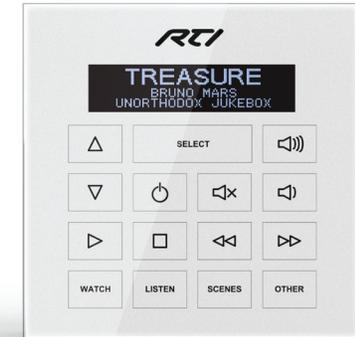
The WK2 Water Resistant In-Wall Controller has a clean, sleek design with an all glass exterior that is perfect in locations such as bathrooms. The solid state glass keypad utilizes capacitive touch for the fourteen programmable buttons. A bright OLED display provides two-way feedback for fast, intuitive control when used with an RTI XP series control processor.
