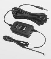
The VPS-1 Voltage Power Sensor monitors the on and off status of almost any electronic component. It is used to provide power status information to RTI control systems such as the RP-6 controller for instance. When the attached component is powered on, the VPS-1 detects the voltage supplied from the component, an attached power supply, or a third-party power sensor, and sends a signal to the RTI controller.
