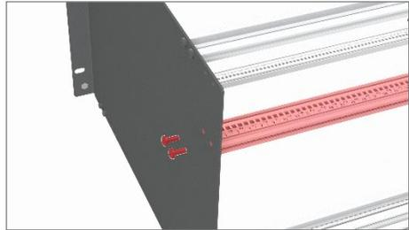
3. Position the upper rail with the numbers facing downwards and the M3 bolt strip facing outwards. Use four M4 screws to connect the rail to the side panels.
