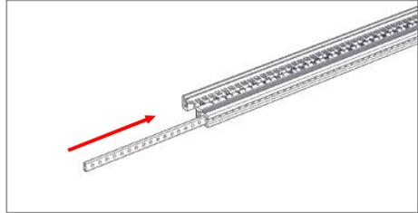
2. Work from the rear of the chassis. Position the lower rail with the numbers facing upwards and the M3 bolt strip facing outwards. Use four M4 screws to connect the rail to the side panels.
