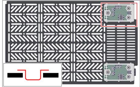
2. Turn the module over and screw the voltage selector in place with three M4 screws.
