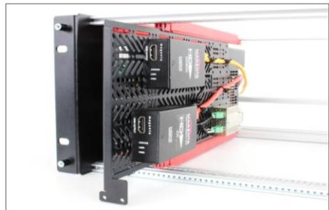
3. At the rear of the chassis, push the dock into the new voltage selector. Use the module to help you align the dock.
