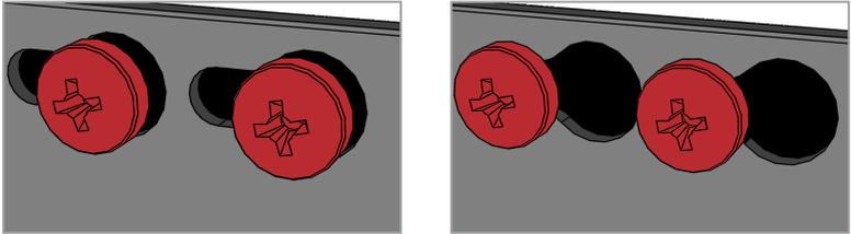
Any screws that don't also hold a mounting rail in place need a nut.
