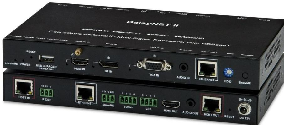
DaisyNET II is a cascable, 4K multiformat extender for various AV signals, Ethernet and control commands. Using HDBaseT technology, DaisyNET II can distribute these signals via a CAT cable (CAT5e, CAT6A, CAT7) over a distance of up to 100 meters from device to device without quality loss or any visible latency.
