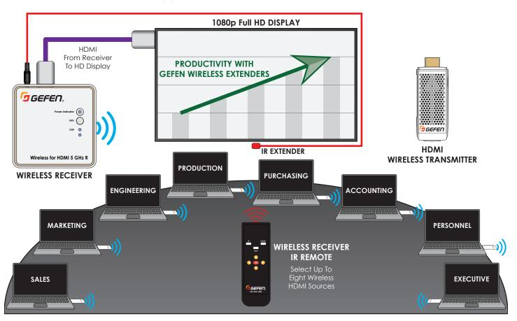
Conference Room application with Wireless Transmitters connected to laptops for a staff meeting. Up to eight Wireless Transmitters can be used to transmit 1080p HDMI to the Wireless Receiver. Laptops can be individually selected with the IR Remote for presentation on the HD Display.
