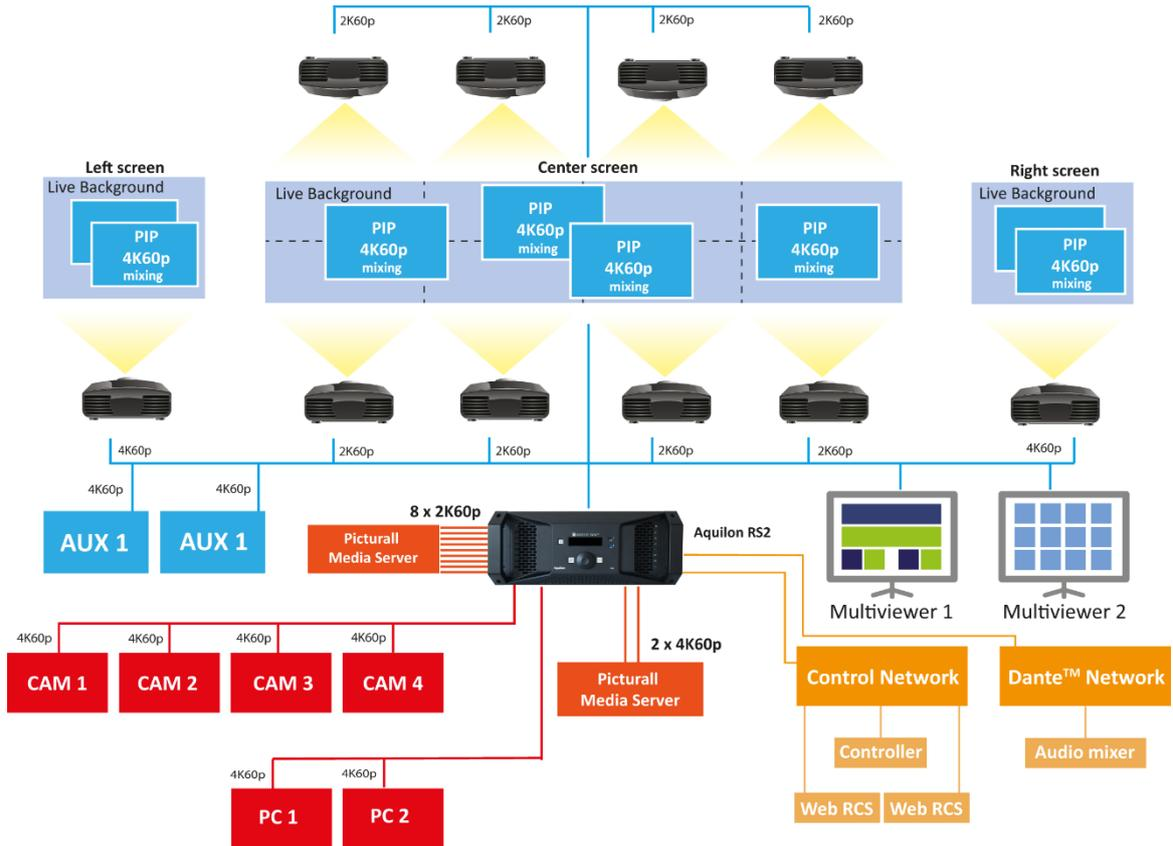
**Aquilon RS2 can drive 2x 8K60p LED walls and 4x 4K60p AUX outputs**
